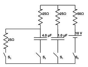
(a, 5) Switches  $S_0$ ,  $S_1$ ,  $S_2$  are closed. Switch  $S_3$  remains open. After a very long time, what is the charge on each capacitor?
